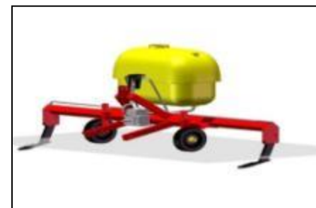
Feeder for applying mycorrhizal preparations under soil surface close to the root system
